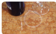
Step 1 Acid based contaminants will etch, eg: wine etch on calcium based stone.
