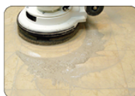
Step 3 Use a weighted slow speed scrubbing machine with hogs hair pad or tan pad.
